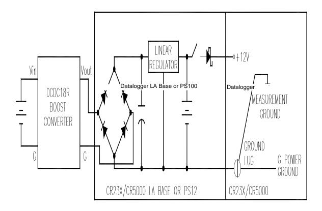
Figure 4. Schematic of Charging and Grounding Circuitry
