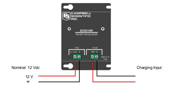
Figure 2. Wiring for DCDC18R
